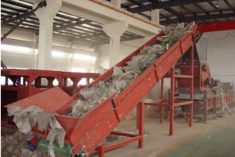
Plastic bags loaded onto a conveyer entering a plastic bag recycling machine.
