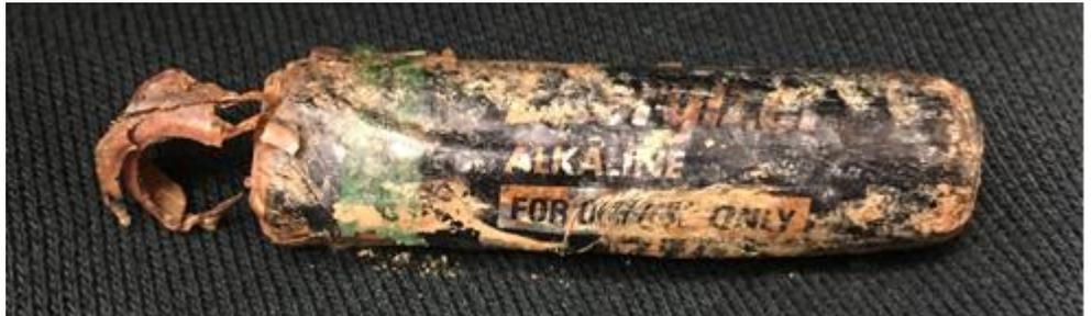
Above: A battery that was recovered from the landfill that has corroded and released its contents.
