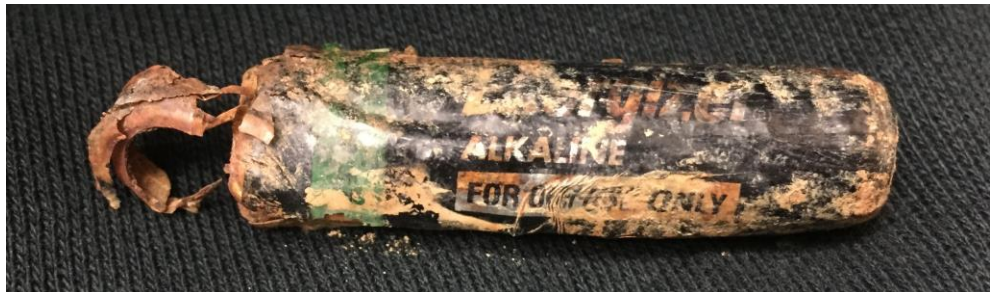
Above: A landfilled alkaline battery that has corroded and released its contents.
